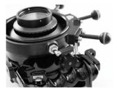
6. Clean the groove where the ring arm mount is placed. When you place back the ring arm mount to the base, please reverse the procedure.
